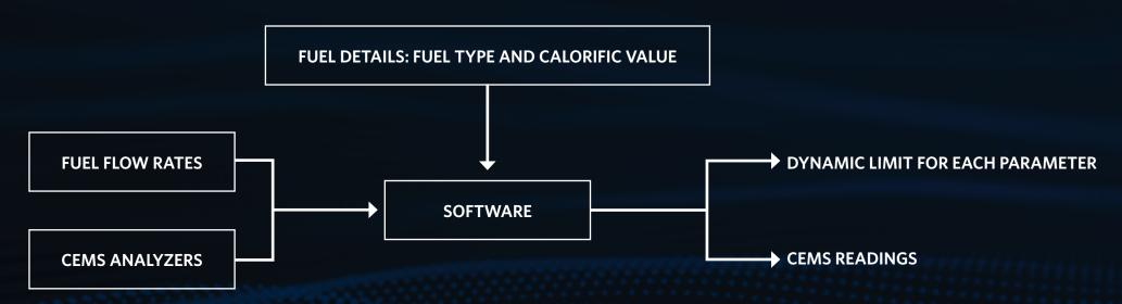
Figure A: Emission Model Conceptual Diagram, \*CEMS Continuous Emission Monitoring System
